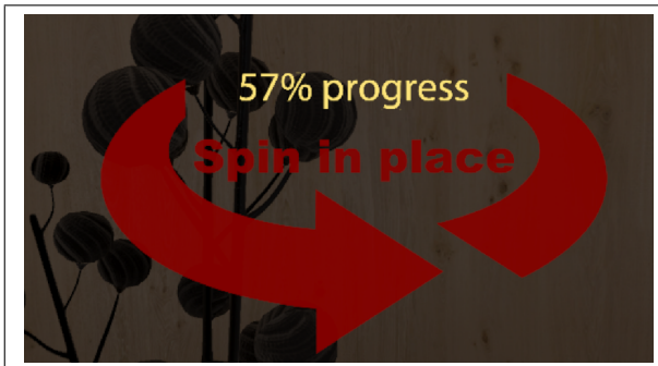
Fig. 4. A screen shot of our “spin in place” warning. Above the rotating arrow, the completion of the turning is shown so that the user knows when she is safe to continue.
